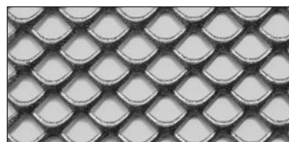
LS10 (Fe) open area 57%, thickness 2.0 mm dimensions: 10 x 7.0 - 1.5 x 1.0 - 1.3 kg/m 2
